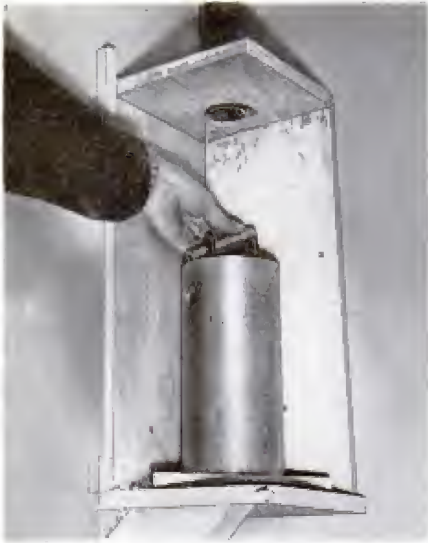
Radioactive sample encased in lead shield fastens at top to cable. Radioactivity is released when . . .
